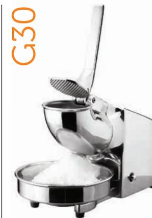
The classic ice crusher to obtain fine ice crystals, to prepare syrup based granitas or refreshing drinks. Light alloy for the motor housing, hopper, lever and blade holder; stainless steel for the crushed ice container and blade. The 300W asynchronous motor with thermal cut-out guarantees continuous duty at any time of day. The safety system, activated by lifting the lever, ensures that the operator works in all safety.
